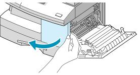
**2** Turn the cartridge locking lever upwards to unlock the toner cartridge, then pull the toner cartridge out.
